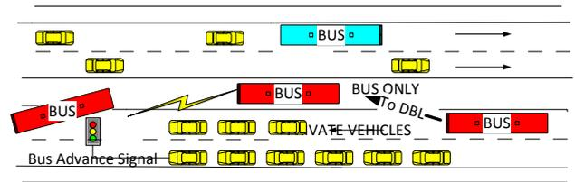
Fig. 6. The Single Dedicated Bus Lane Scenario in the Middle of the Road with Bus Advance
