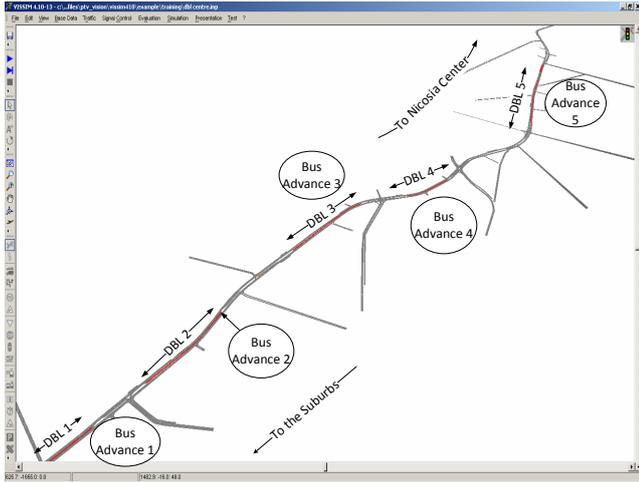
Fig. 3. The Traffic Simulation model showing potential regions for dedicated bus lanes and bus advance areas.
