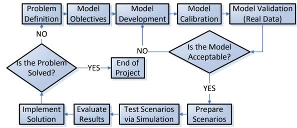
Fig. 2. Proposed Traffic Modeling and Simulation Method
